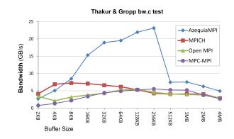
*Figure 5: Bandwidth measurements of four MPI implementations the setup at the right side of Fig. 3.*
