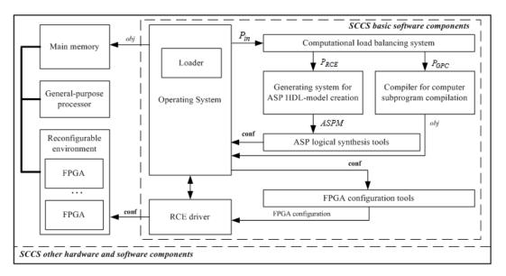
Figure 2: The structure of the self-configurable computer system.
