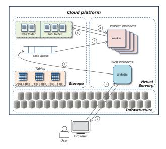
Figure 1: System architecture and application execution steps.
