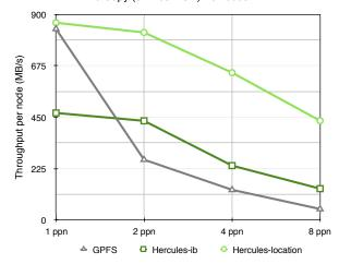
Figure 7: Raw file write throughput per node comparison between our proposed solution and GPFS scaling the number of workers per node running in a fixed 8-node setup.
