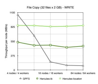
Figure 5: Raw file write throughput per node comparison between our proposed solution and GPFS, when scaling the number of nodes, running one worker per node.
