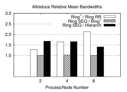
Figure 6: All reduce relative mean bandwidths (calculated for the whole range of messages) of the Ring\* algorithm with respect to the Ring with round robin mapping, of Ring with sequential mapping with respect to Ring\*, and of Ring\* with respect to the hierarchical implementation. All the tests are executed with M = 8 nodes and Q = 8 processes by node, for a total of P = 64 processes.
