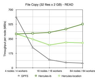
Figure 6: Raw file read throughput per node comparison between our proposed solution and GPFS, when scaling the number of nodes, running one worker per node.
