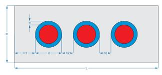
Figure 1: 2D geometry of benchmark problem: three cables in the soil.
