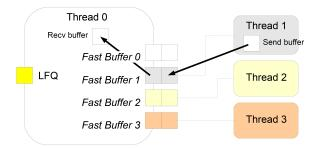
Figure 2: FastBuffers in a configuration of four threads.
